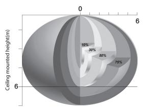
Ceiling mounted detection pattern (m)
