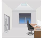
After hold-time, the light dims to Light switches off automatically stand-by level preset.
